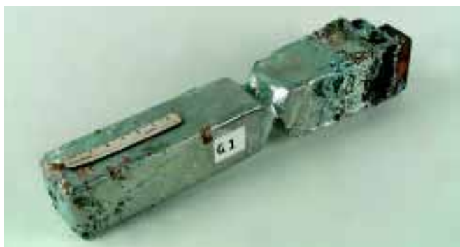
Figure 5. Liquid zinc attack on GMAW weld
