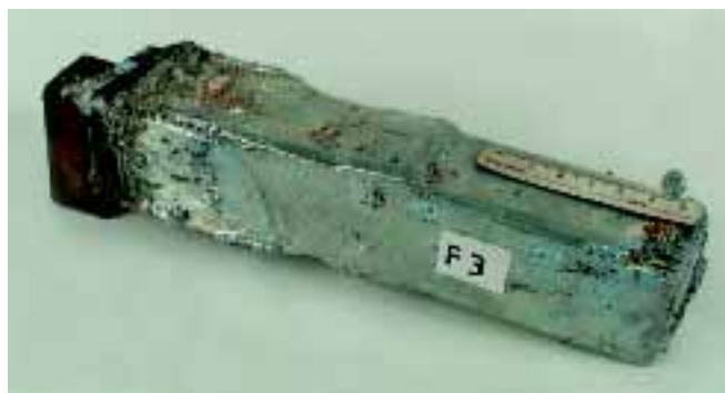
Figure 6. Sample typical of FCAW and MMAW welds after 1 month exposure to liquid zinc
