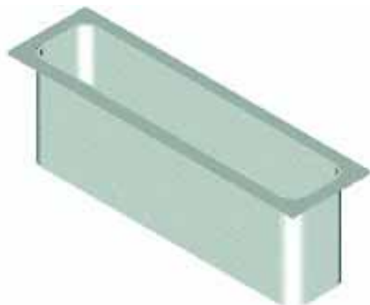
Figure 1. Typical shape of a galvanizing kettle.
