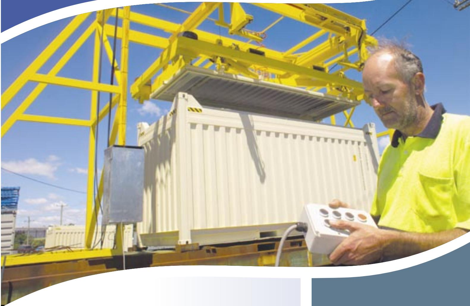
“In tests conducted by BHP Billiton our container was found to carry more product than any others, without exceeding the maximum allowable gross weight limit. We used 350 Grade XLERCOIL® steel in 3mm and 5mm thicknesses to fabricate structural elements of the containers which measure six metres in length, 2.4 metres in width and nearly three metres in height.
