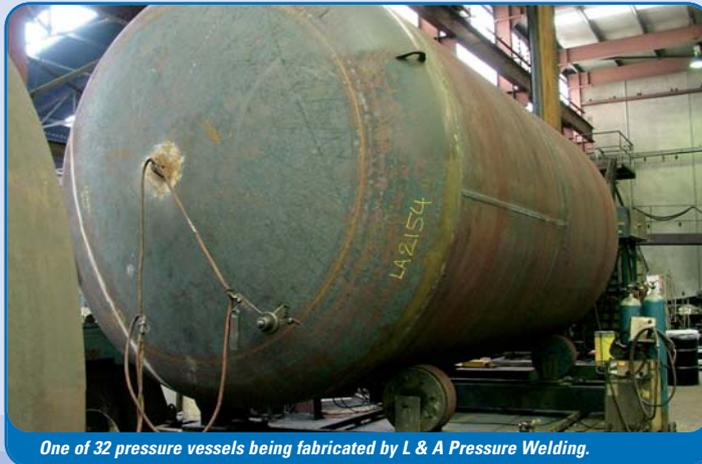
One of 32 pressure vessels being fabricated by L & A Pressure Welding.
