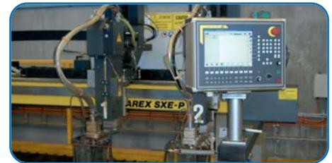
wet-bed machines,” Mr McCarthy said. “It can pierce and cut thicknesses ranging from 3mm to 32mm, and sidecut up to 50mm.”
