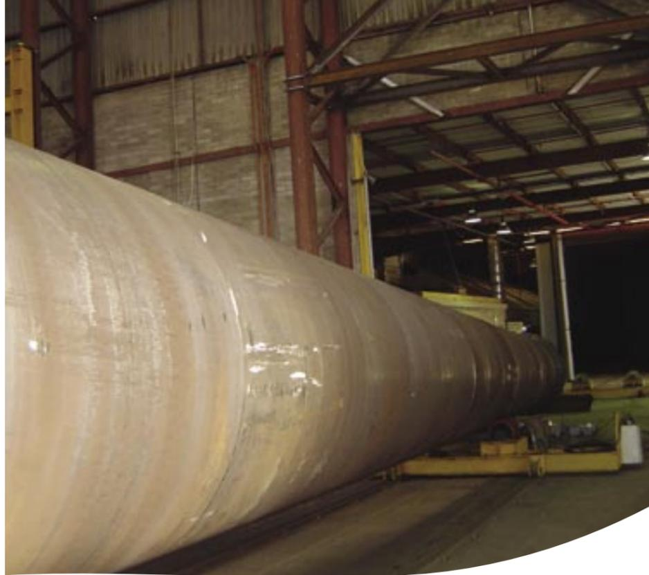
*“In contrast to concrete, a steel pier can be erected in about two hours, with no formwork, shuttering, or scaffolding. So the use of steel, in this case, is a quicker erection method – it minimised time on site, exposure to bad weather and therefore risk.”*
