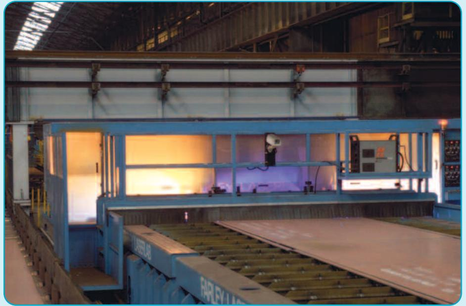
A new plasma cutter is now undergoing final commissioning trials at Port Kembla, providing an extra dimension of efficiency at the Plate Mill.
