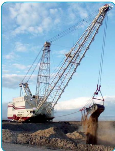
tonnes and wielding a bucket capacity of 89 cubic metres. Its construction has involved the use of nearly 3000 tonnes of XLERPLATE® steel from BlueScope Steel.
