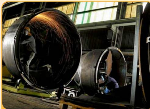
CESCO fabricates mixer barrels made from XLERPLATE® steel.
