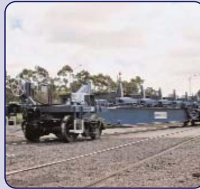
The first of 12 new purpose-built tilt rail wagons, designed to carry wide XLERPLATE® steel across Australia, have entered service.
