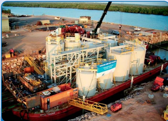
EC&E shipped the Milk of Lime Process Tanks to the refinery.
