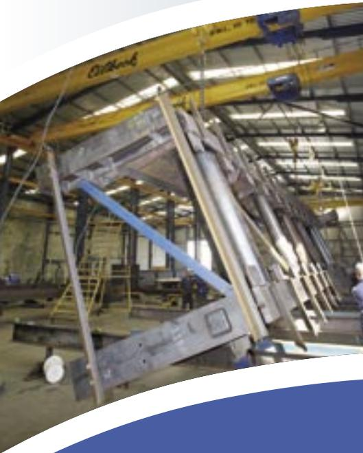
“At that stage, multiple checking procedures were carried out to ensure dimensional accuracy, weld preps and so on. We tried to produce the structure in as small components as possible, prior to assembling the whole unit.
