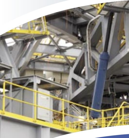
Which is why they chose XLERPLATE® steel, a brand of high quality hot-rolled steel from BlueScope Steel. 800 tonnes of 350 grade XLERPLATE® steel was used in the ship loader's fabrication.
