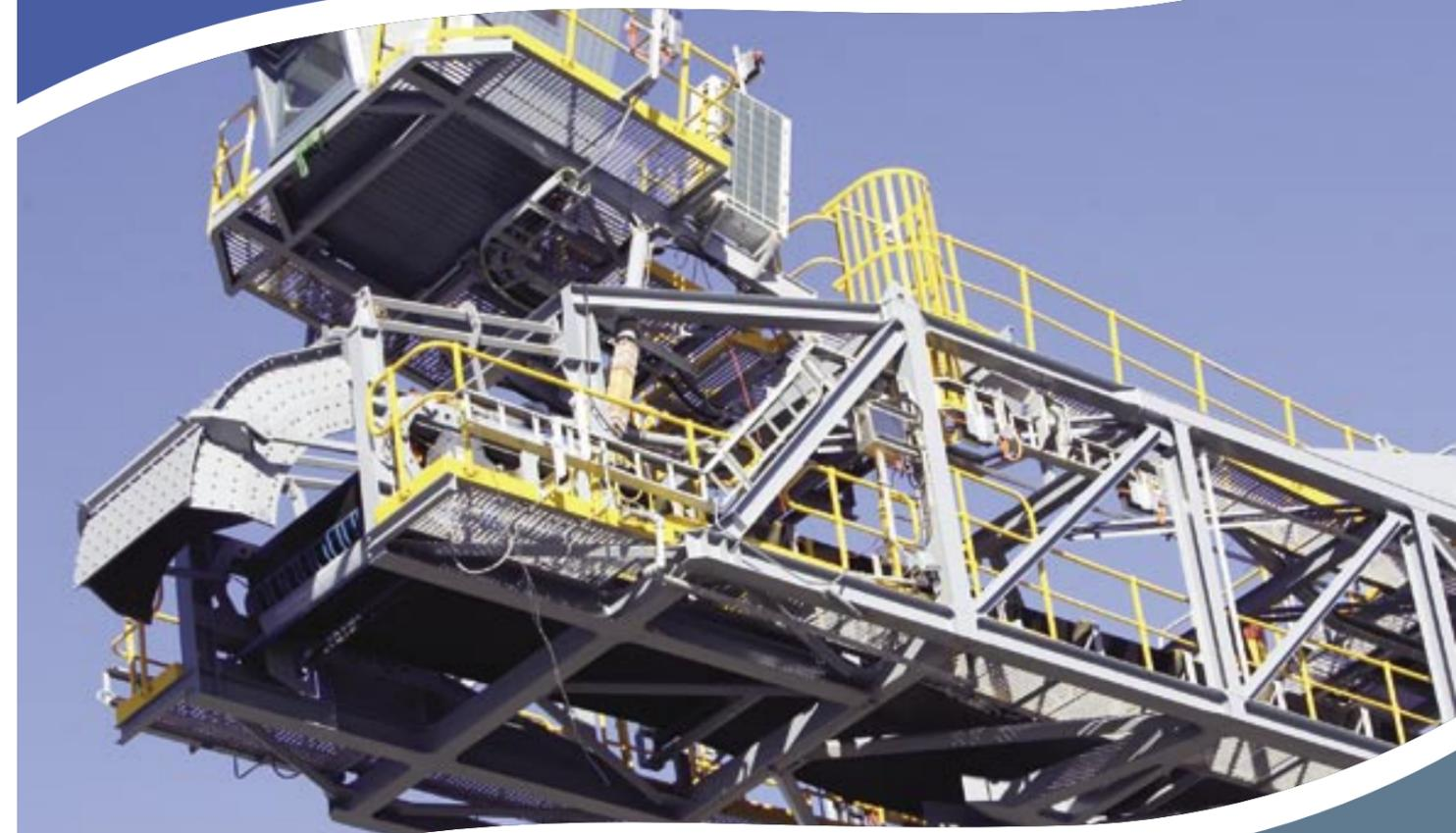
The overall length of the ship loader is 112 metres. The boom is 52 metres from the tip to the centre, and the loader stands 28 metres high. Fully assembled, the machine weighs 900 tonnes.
