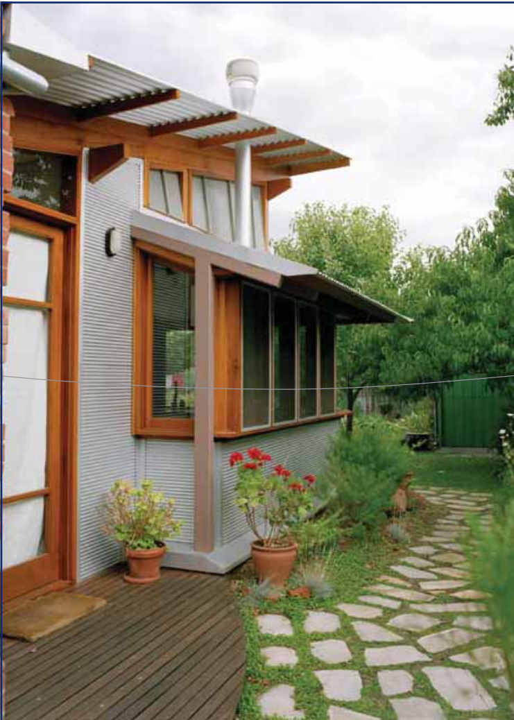
The Nobbs Blyfield development in Maylands, South Australia added a contemporary and environmentally-friendly backyard extension to a 1900s inner suburban villa. Troppo Architects chose framing, roofing and wall cladding made from BlueScope Steel's ZINCALUME® steel for the home extensions.
