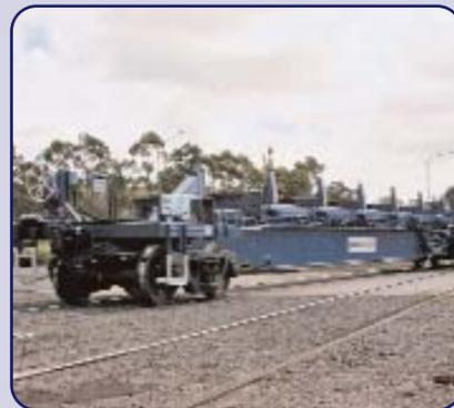
The first of 12 new purpose-built tilt rail wagons, designed to carry wide XLERPLATE® steel across Australia, have entered service.
