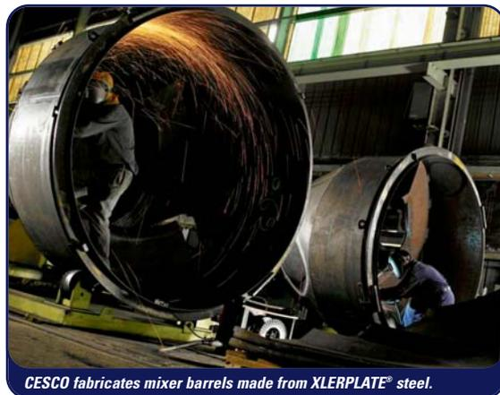
CESCO fabricates mixer barrels made from XLERPLATE® steel.
