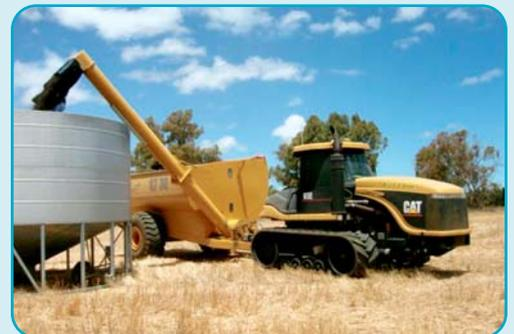
reach discharge augers allow for fast unloading rates.
