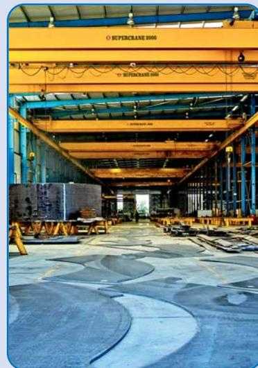
workshop floor space by 3000 square metres and added four new cranes. We designed the cranes ourselves, then built them using 150 tonnes of XLERPLATE® steel.
