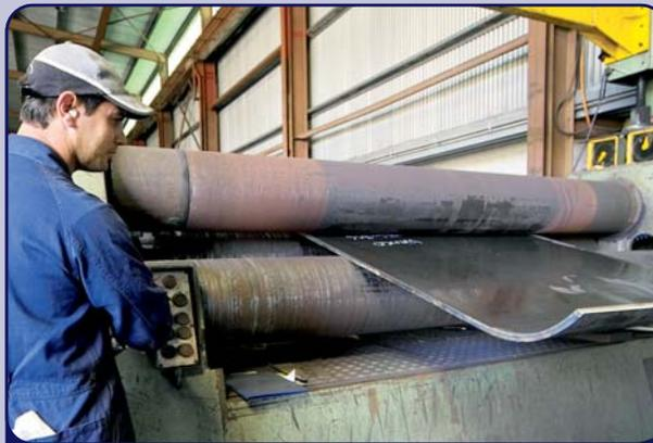
Inside the Wenco workshop where outer dome plates are being fabricated.
