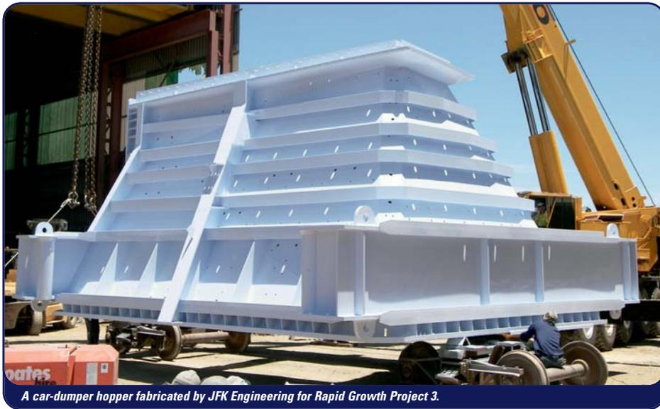
A car-dumper hopper fabricated by JFK Engineering for Rapid Growth Project 3.
