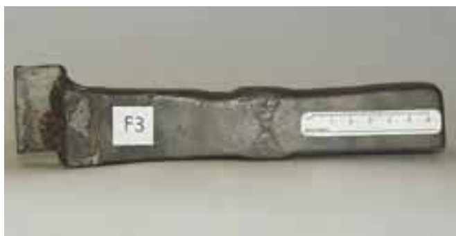
Figure 7. Typical sample after 12 months exposure to liquid zinc.
