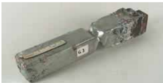
Figure 5. Liquid zinc attack on GMAW weld after 1 month.
