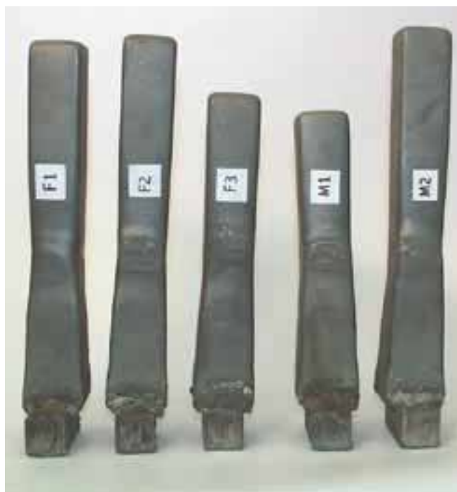
Figure 8. Profile view of the long term test pieces from the continuous kettle, showing wasting.
