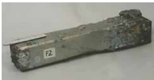
Figure 6. Typical sample after 3 months exposure to liquid zinc.
