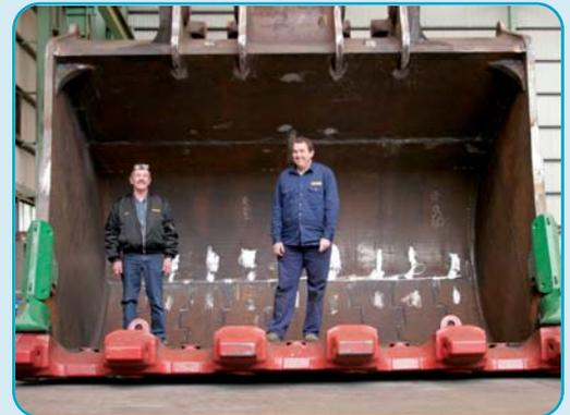
then machined to take bushes which are shrink-fitted using liquid nitrogen," Mr Lankowski said. "The bearing block area is stress-relieved before being fitted to the bucket because of the amount of welding we perform."
