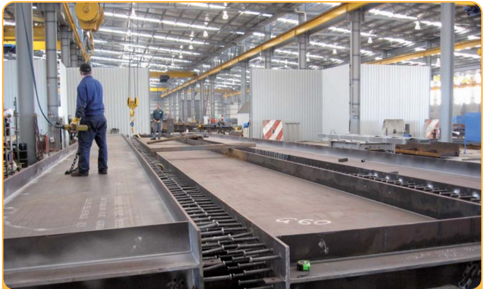
Rail bridge girders in Samaras Structural Engineers’ workshop.
