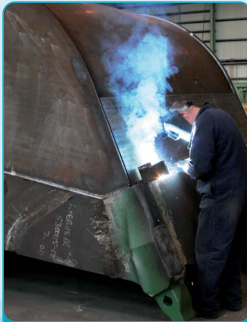
Welding XLERPLATE® steel in Liebherr-Australia's workshop.
