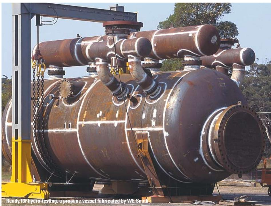
Ready for hydro-testing, a propane vessel fabricated by WE Smith.
