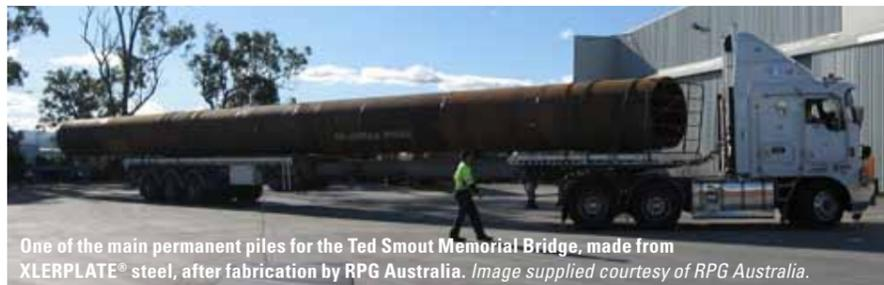
One of the main permanent piles for the Ted Smout Memorial Bridge, made from XLERPLATE® steel, after fabrication by RPG Australia. Image supplied courtesy of RPG Australia.
