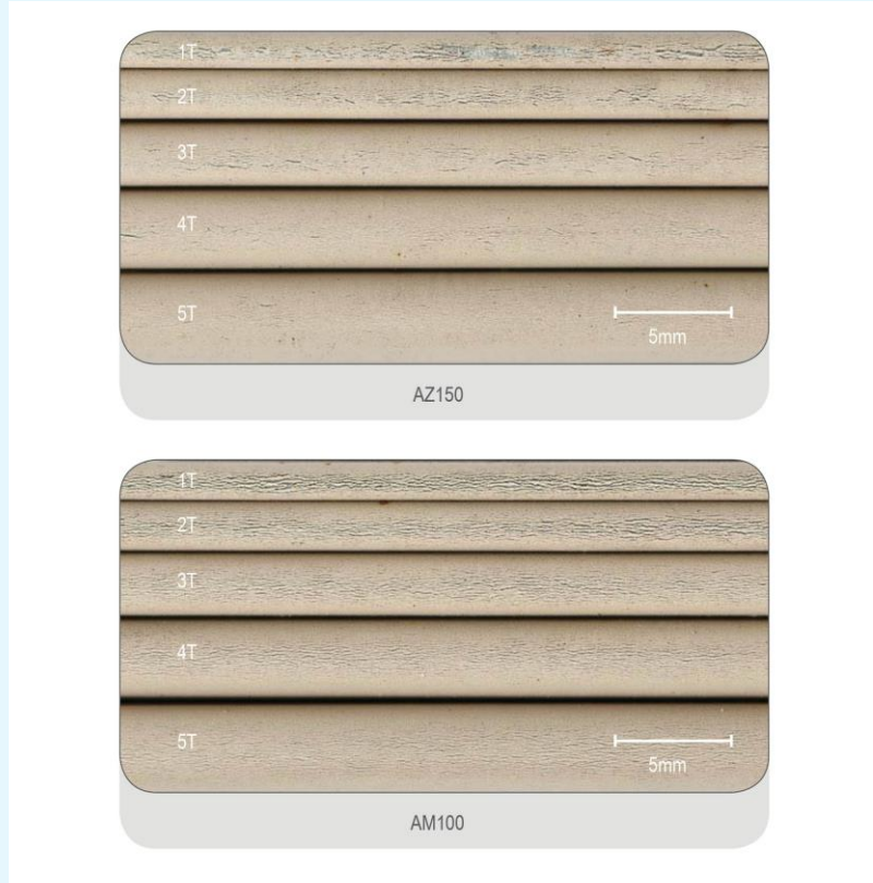
Figure 8: Prepainted bend samples exposed in an unwashed marine environment for 51 months.
