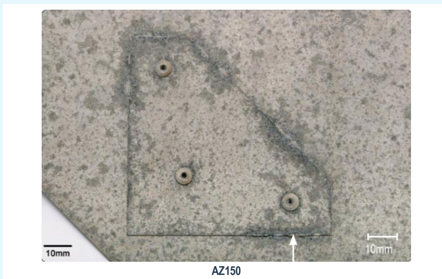
Dark areas indicate metallic coating corrosion originating from the cut-edge.
