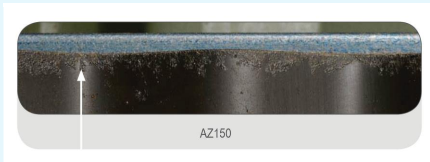
Blisters developed from cut-edge protection.
