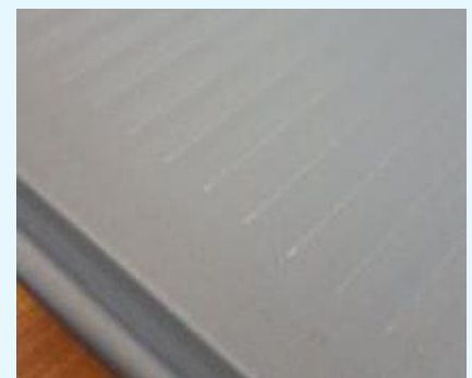
Figure 1: Pressure marring is visible on this formed section of COLORBOND® steel as glossy lines on the ribs and bends
