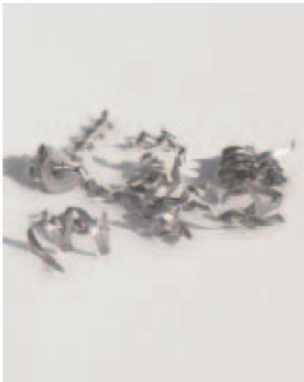
Ensure all swarf (drill waste) is removed from the work area.
