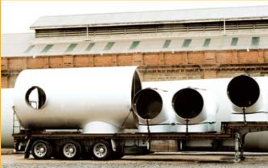
Air Ride Wind has fabricated five hot-air ducts and a section of the stack for the new walking beam reheat furnace. Mainteck Services, a Port Kembla-based construction company contracted to part-manufacture and erect the new furnace, approached Air Ride Wind to undertake the work.
