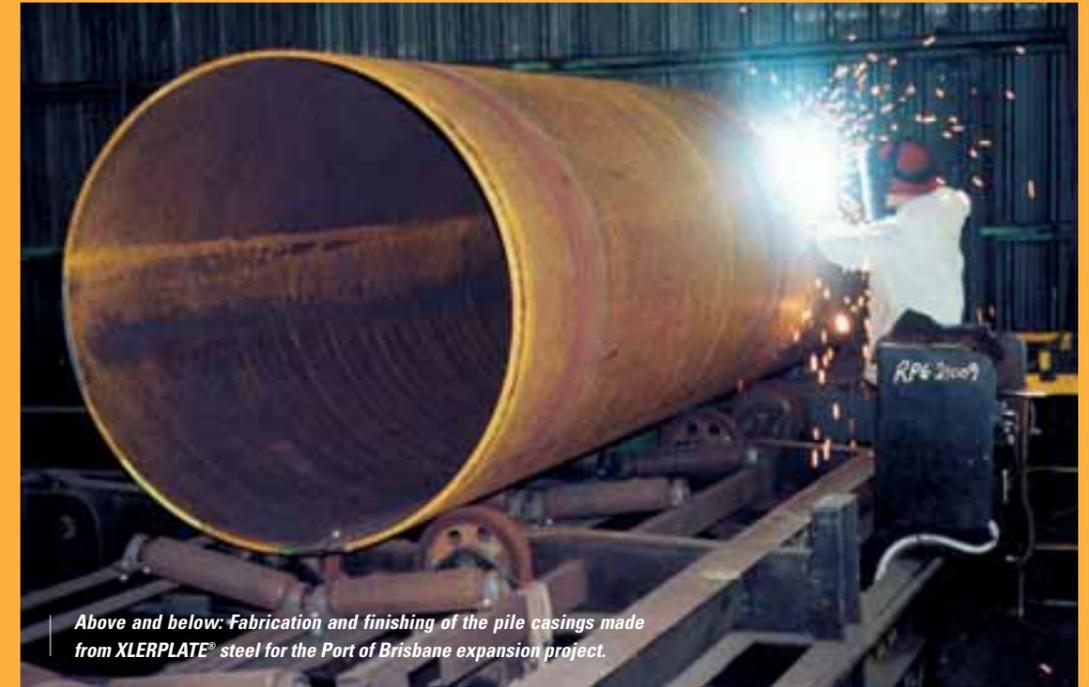
*Above and below: Fabrication and finishing of the pile casings made from XLERPLATE® steel for the Port of Brisbane expansion project.*
