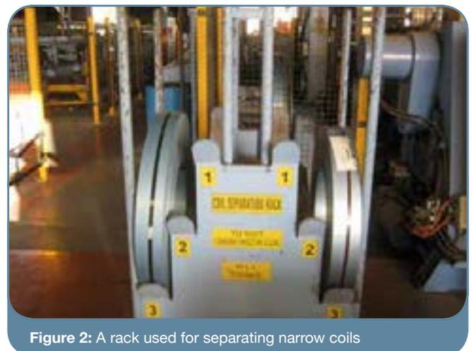
Figure 2: A rack used for separating narrow coils
