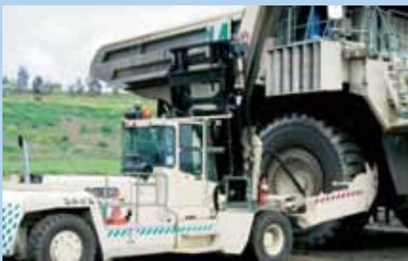
The Omega Tyre Handler, made from Grades 250, 350 and 400 XLERPLATE® steel in thicknesses ranging from 5mm to 160mm, is one of a number of local product innovations from Clark Equipment – a company often associated with small forklift trucks.
