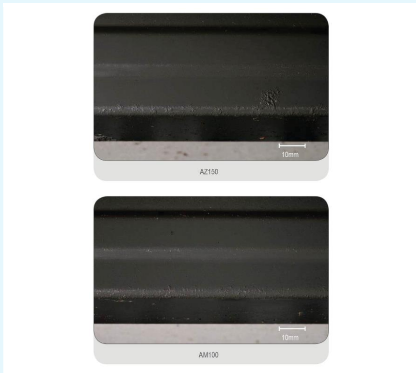
Figure 7: Prepainted, sheltered fascia bends (i.e. unwashed) after 57 months exposure within 100m from breaking surf on an outdoor test facility.
